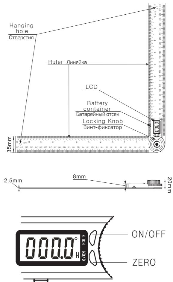
**ON/OFF** Short press ON/OFF to turn on the device. Short press ON/OFF to shut off the LCD. Long press ON/OFF for more than 3 seconds to shut off the whole system. Automatically shut off function in 6 min. Move the scale to turn on the device when at off LCD status.
